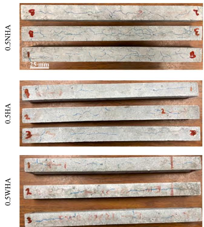
Fig. 14. Cracks developed on the surfaces of mortar bars under ASR conditions.
